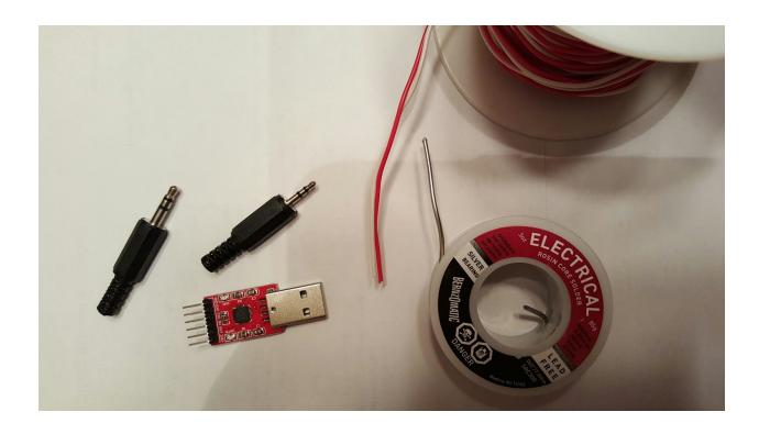
The 2.5 mm plug ground goes to the ground on the CP2102. The 2.5 mm plug TX Data goes to the receive data on the CP2102. The 3.5 mm plug Mic/RX Data/PTT goes to the transmit data on the CP2102. The RX and TX connections may need to be swapped based on the CP2102 version you get. Don't tie things down until you test it.
